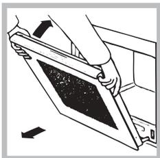
3. Grip the door on the two external sides and close it approximately half way. Unlock the door by pressing on the clamps **F**, then pull the door towards you lifting it out of its seat (*see diagram*). To replace the door, reverse this sequence.
